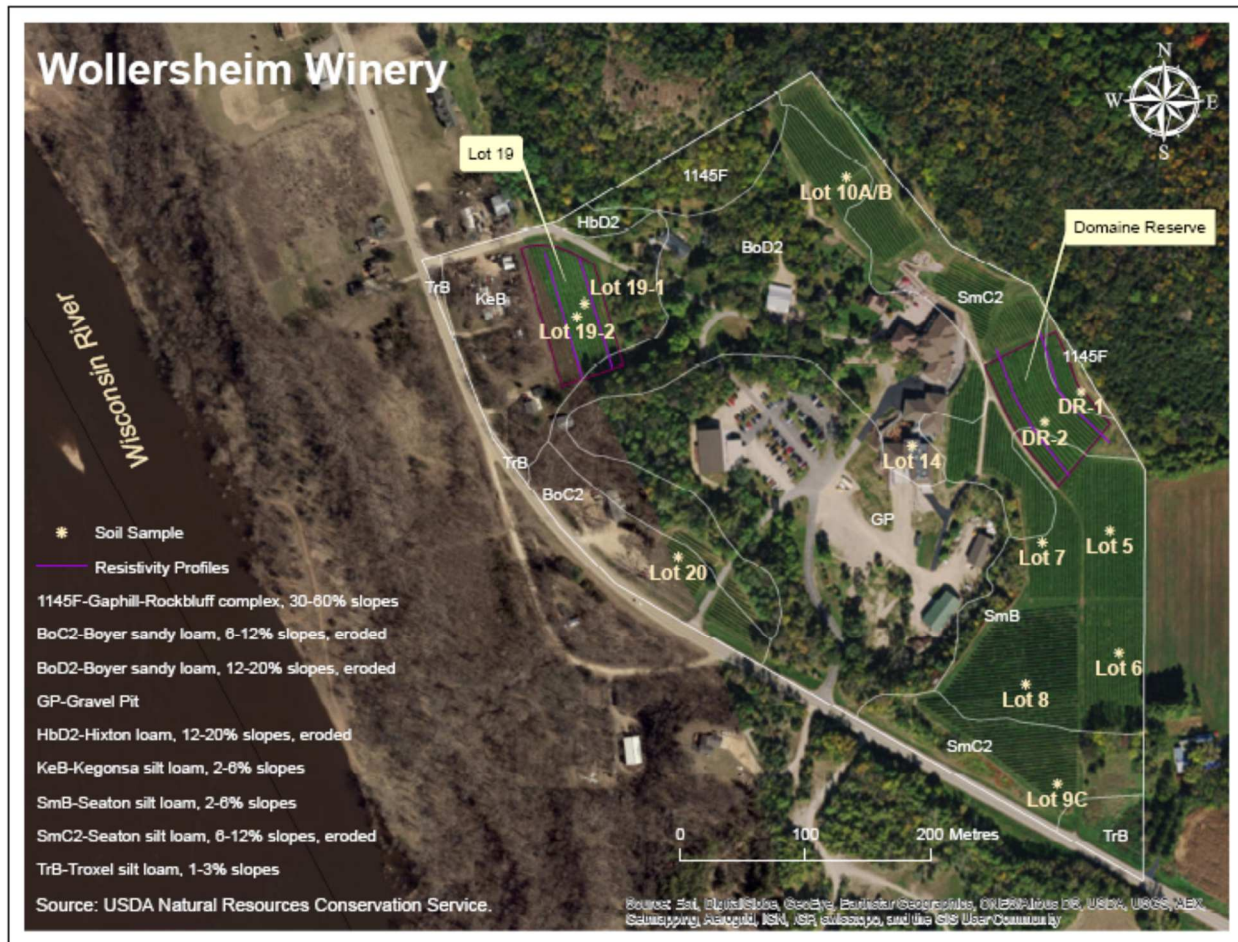
Figure 2-4. Location map of Wollersheim Winery vineyards illustrating the distribution of soil types, and soil sample and resistivity profile locations.
